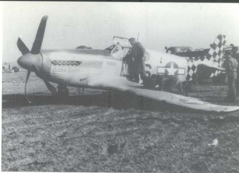
BOSS BABY, number 86, was another Mustang that suffered a hydraulic failure and suffered damage as a result of a failed main landing gear leg. The aircraft was flown by Lieutenant Harry S. Carroll of the 319th Fighter Squadron. (Checkertail Clan)
