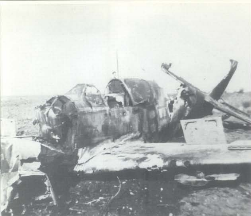
SOCKO , a P-51C, number 78, of the 319th Fighter Squadron crashed and burned. The crash crews have opened the ammunition bays to make sure that all unexploded ammunition has been removed from the wreck. (Checkertail Clan)
