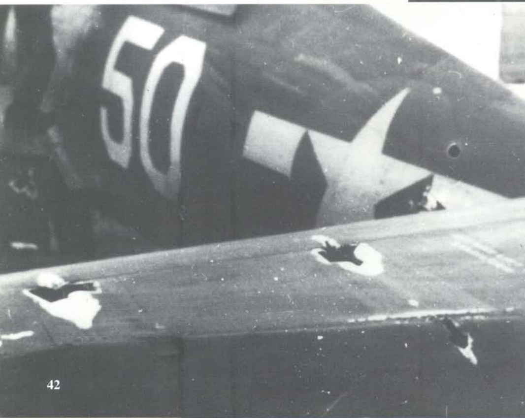
(Above and Left) Butch, number fifty of the 318th Fighter Squadron was assigned to Lieutenant L. W. Adams and crewed by SGT William Stolarczyk. The aircraft was shot up by an enemy fighter on a mission and had large pieces shot out of the wing, starboard elevator, and port horizontal stabilizer/elevator. Much of the damage was actually minor in nature, being mostly sheet metal work with little internal damage. This sequence proves the ruggedness of the Thunderbolt. The P-47 had a well deserved reputation of being able to withstand a lot of battle damage and still get its pilot home. (William Stolarczyk)
