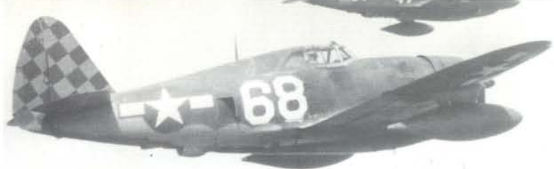
Lieutenant Chester L. Williamson flew as wingman for Lieutenant Benjamin Emmert. The underwing tanks on this P-47D are actually P-38 drop tanks. The underwing pylon on the Thunderbolt was locally modified to accept these large streamlined tanks, replacing the bulky underfuselage tanks issued with the P-47. (Checkertail Clan)
