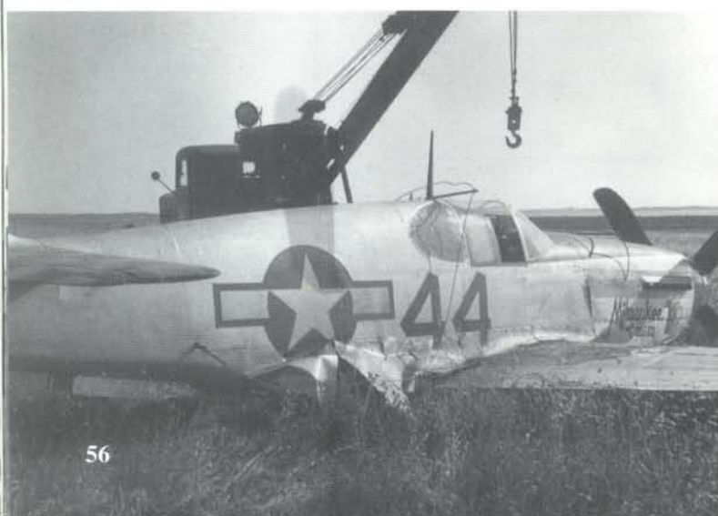
The salvage crews are ready to lift Lieutenant Dowd's Mustang and cart it off. The damage to the belly scoop was quite evident and it was doubtful that this Mustang would ever fly again. (Paul Dowd)
