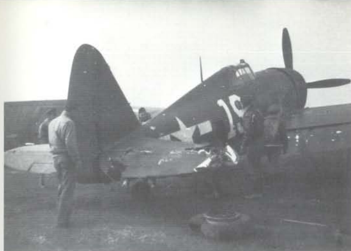
This P-47D of the 317th Fighter Squadron was shot up by ground fire, but was able to make it back to base in spite of severe damage to the tail. (Checkertail Clan)
