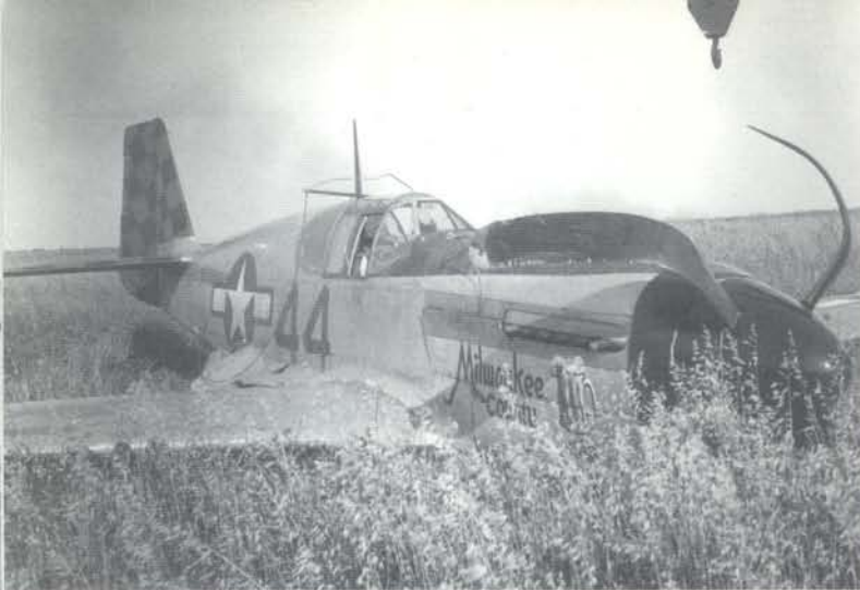
Lieutenant Paul Dowd crash landed in Milwaukee County. The aircraft came to rest in a field after it struck a ditch off the end of the runway and sheared off the landing gear. The propeller was still turning when the gear ripped away as is evident by the bent blades. (Paul Dowd)
