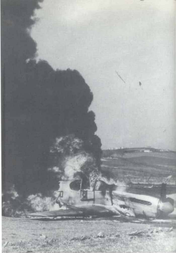
This unidentified P-51 on fire in the middle of the field seems to have made a power-on belly landing as indicated by the bent propeller blades. (Checkertail Clan)
