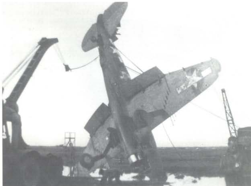
Salvage crews use several mobile cranes to right number 49 and place it back on its landing gear. Once the aircraft was righted, it could be towed back to the squadron area for a detailed assessment of the damage. (William Stolarczyk)
