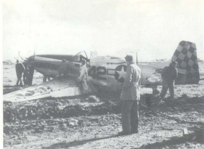
Number 42 made a crash landing and had the main landing gear fail. It was just one of many to suffer this type of accident. (Checkertail Clan)
